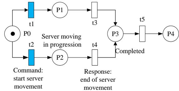
Fig. 3. Scenario of server movement in PN-based repair subsystem using the command/response concept
