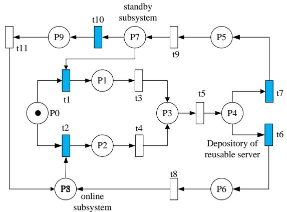
Fig. 4. PN-based framework design on the proposed system
